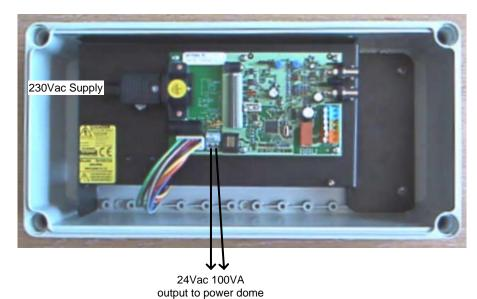
**Important!** When operating the unit from 24Vac, the fuse from 230Vac the connector fuse holder must be removed. No connections must be made to this connector, as it will have 230Vac across the L & N terminals.
